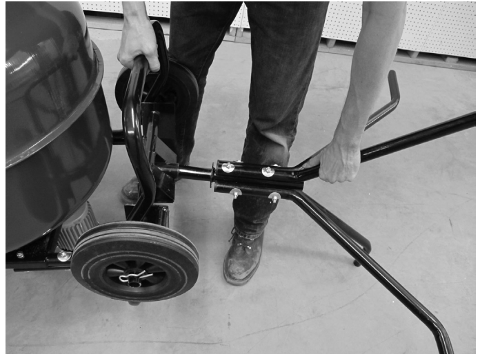
Lift mixer slightly and insert pedestal.
