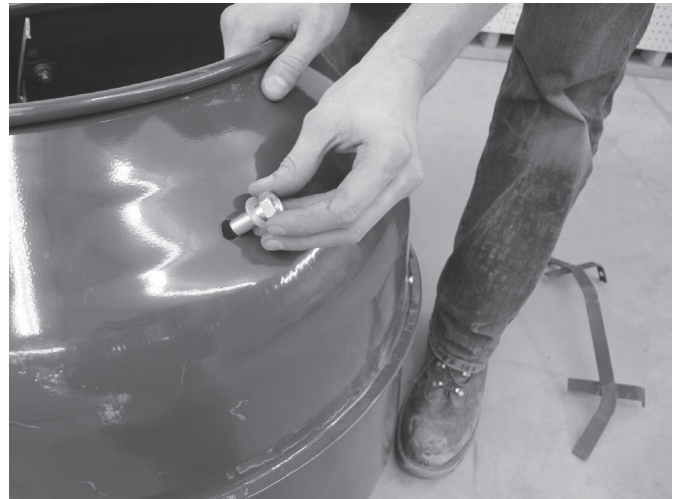
Insert bolts through drum.
